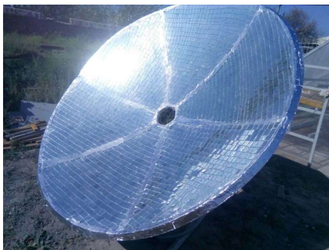
Fig. 3 Appearance of the fabricated parabolic concentrator
